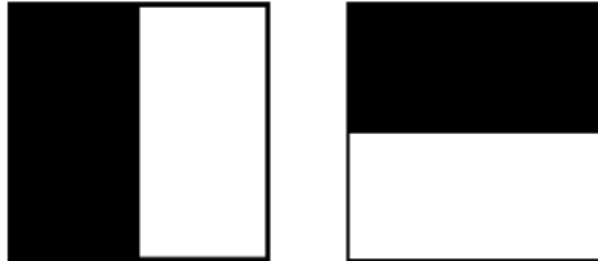
Fig. 8. Haar wavelet filters to compute the responses in x (left) and y direction (right). The dark parts have the weight -1 and the light parts +1.
